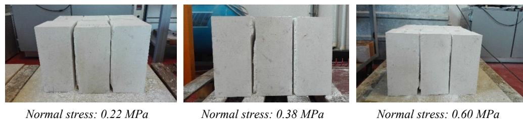
Figure 8. The observed failure modes of triplets for different axial preloads.
