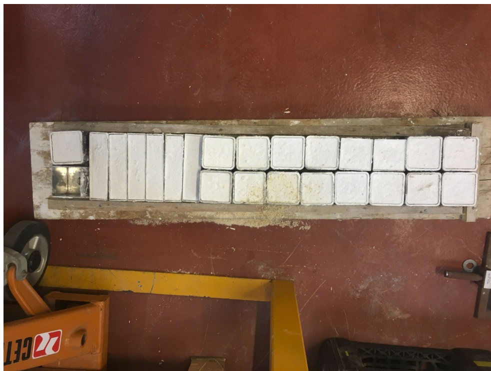
Figure 4. The mortar specimens manufactured for compression and bending tests.
