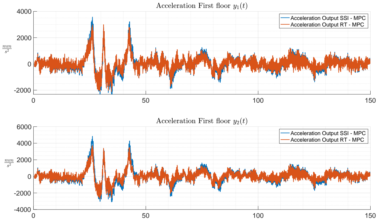
FIGURE 13 Top: acceleration comparison of RT-MPC and SSI-MPC for the first floor. Bottom left: acceleration comparison of RT-MPC and SSI-MPC for the second floor
