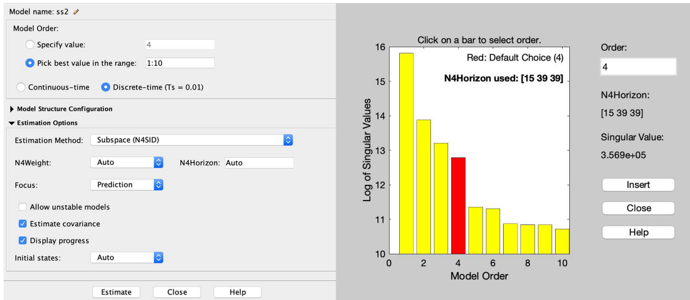
FIGURE 4 Matlab System Identification Toolbox APP. Some settings used to derive LTI models
