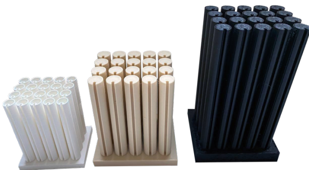
Figure 3 - Scaled prototypes of 3D printed Sonic Crystal Noise Barriers
