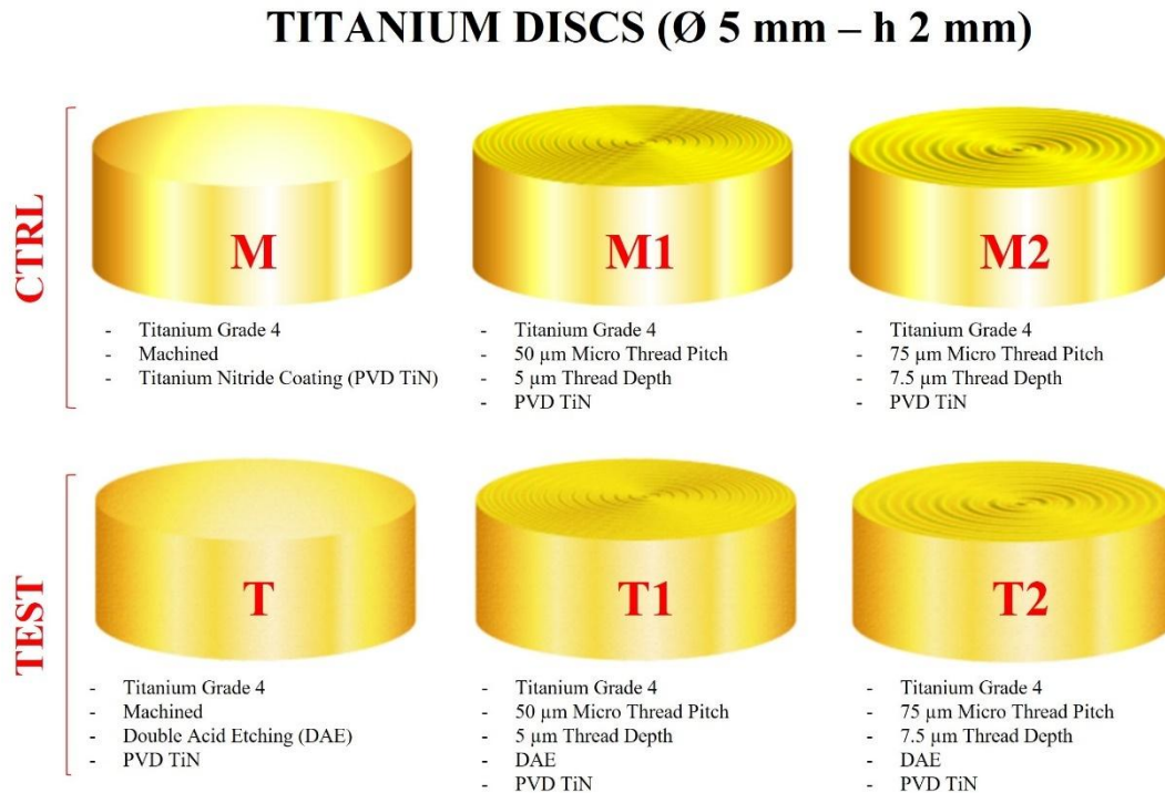
Figure 7. Schematic illustration of the characteristics of the surfaces under analysis. The discs were divided into six groups based on their surface treatments and micro-morphologies: machined (M); with 50×5 µm threading (M1); with 75×7.5 µm threading (M2); and their corresponding treated surfaces undergoing a double acid etching (DAE)
