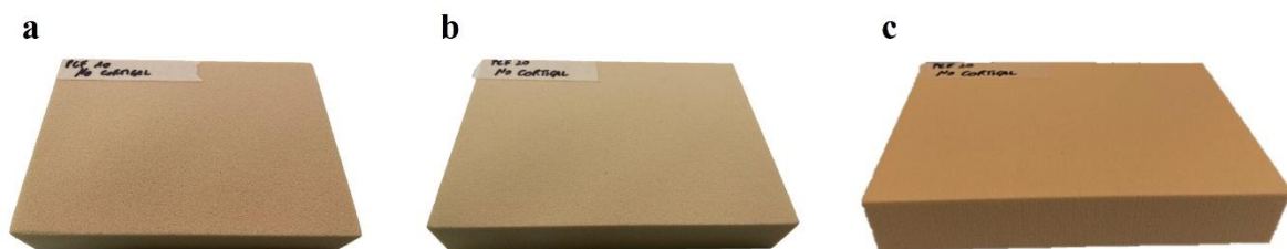
Figure 45. Solid rigid polyurethane foam blocks used in the present study. (a) A block with a density of 10 pounds per cubic foot (PCF); (b) A block designated as 20 PCF density; and (c) A block designated as 30 PCF density.
