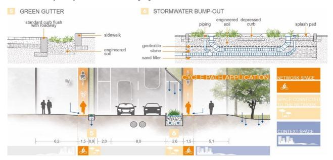
**Figure 14:** Philadelphia, section and planimetry of Green Gutter and Stormwater Bump-Out: a hypothesis of application to the cycle path. *Original drawing by arch. Angelica Nanni*.
