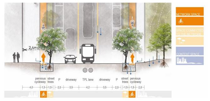
Figure 6: Melbourne, section and planimetry of La Trobe Street green bicycle lane. Original drawing by arch. Angelica Nanni.
