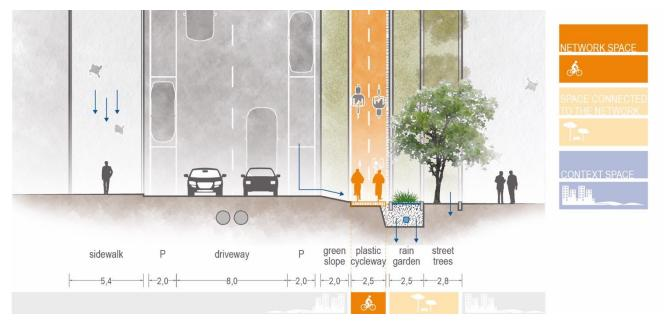
Figure 7: Zwolle, section and planimetry of Plastic Road in Deventerstraatweg. Original drawing by arch. Angelica Nanni.
