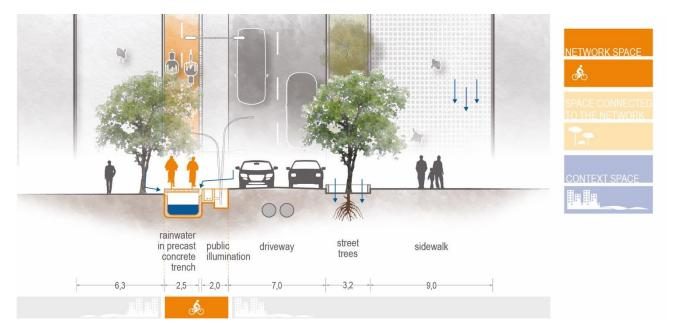
**Figure 9:** *The Copenhagenize Current* the design project for a prefabricated canal below the cycle path by Mikael Colville Andersen and Steve Montebello. *Original drawing by arch. Angelica Nanni*.
