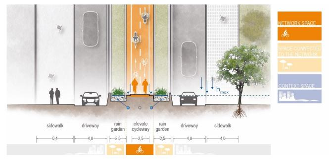
Figure 5: San Rafael, section and planimetry of Canal Street. Original drawing by arch. Angelica Nanni.
