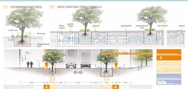
Figure 13: Philadelphia, section and planimetry of Stormwater Tree and Infiltration Tree Trench: a hypothesis of application to the cycle path. *Original drawing by arch. Angelica Nanni*.
